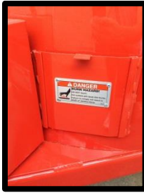
Figure 5.5 Propane Burner Access Door
