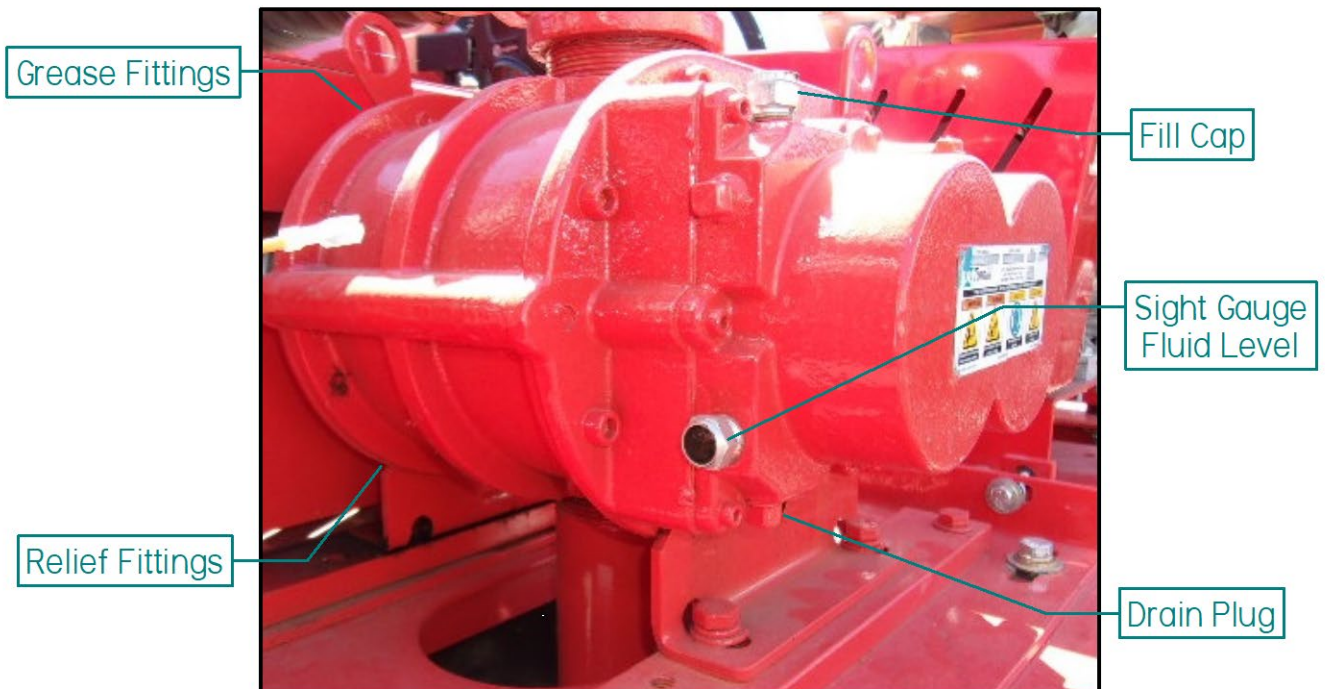
Figure 5-2 Rotary Blower Fluid Level
