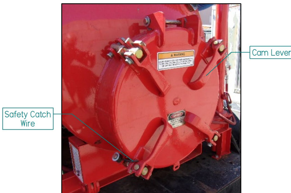
Figure 5-7 Debris Storage Tank Door
