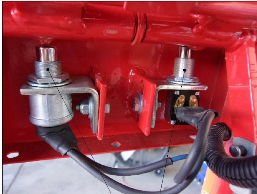
Figure 6-12 Self-Propelled Safety Cutoff Switch
