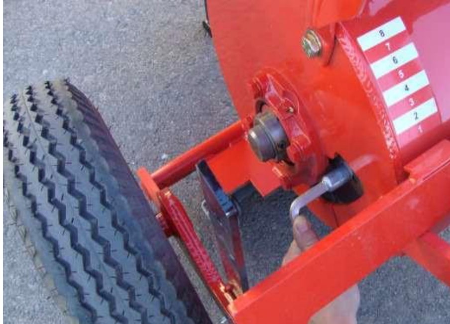
Figure 6-4 Wrench in Cutter Window
